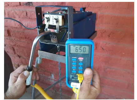
Pyrometer indicating proper blade temperature of 650°C.
